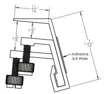
Bracket can be adapted to shelf thickness by changing clip from short side to long side.
